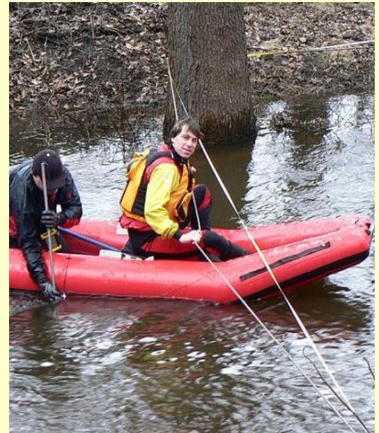
Photo: T.Vránek, 2009 Hydrometry on Dračice River B-order hydrological profile: stream measurement for river system evaluation project within the frame of the Czech Ministry of Environment program
